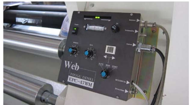
Controller Series 47 is installed on Rewinding Machine
